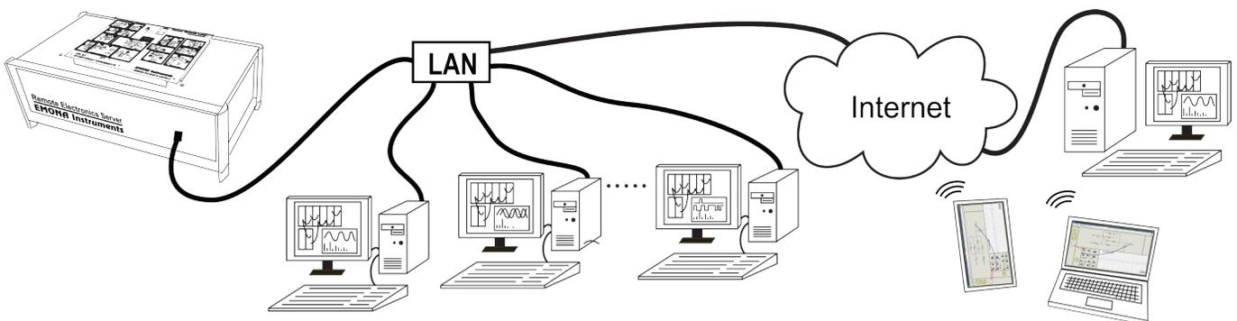
netCIRCUITlabs experiment accessible via LAN and Internet using PC, laptop and tablet web browser.
