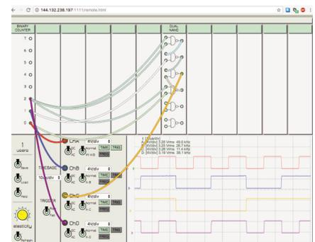
Example of a wired 2 input Multiplexer
