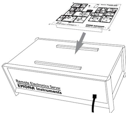
netCIRCUITlabs Control Unit connects router, hub or LAN. Lab Experiments board shown not plugged-in.
