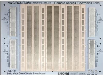
1. Large 2,692 point solderless breadboard with distribution strips and component breadboarding area.
