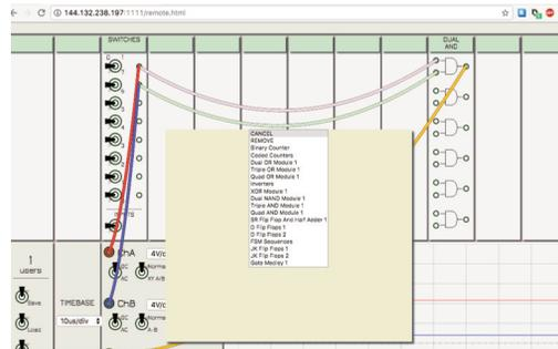
Students build digital logic experiments by selecting and patching real logic gates and functions. Over 60 independent elements are provided.
